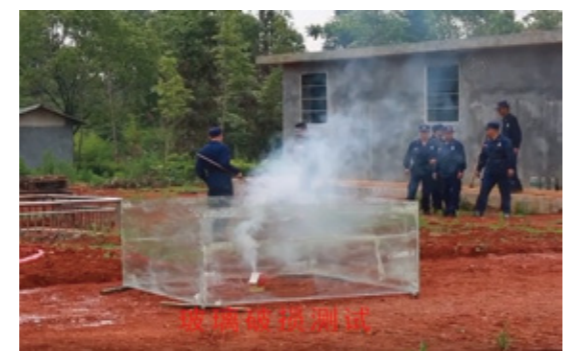
The fire extinguisher device would not damage the 0.5cm glass
