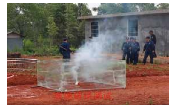
The fire extinguisher device would not damage the 0.5cm glass
